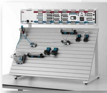
**Example's of Festo Didactic components that competitors may use to design, build and test the function a Multi Cylinder Sequential or Cascade Circuit that may include time-delay, flow control and / or check valves.**
